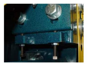
2) Take the two jacking bolts per side as seen above and snug them just to the point you can't get a .002" shim or a standard piece of paper between the blade holder and the brass in all four points (as seen below).
