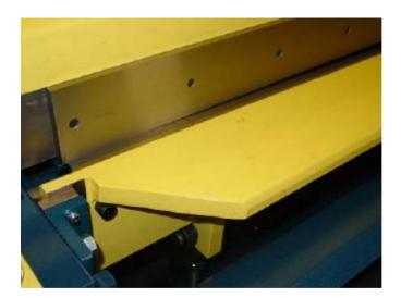
2) Starting with the high side, match the cutting edges as seen in the pictures below. Adjust the top blade by using jacking bolts to the point of both blades touching.
