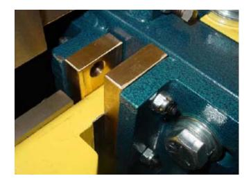
\*As you operate the shear over time, the brass with normal wear can allow the blades to become out of adjustment.
